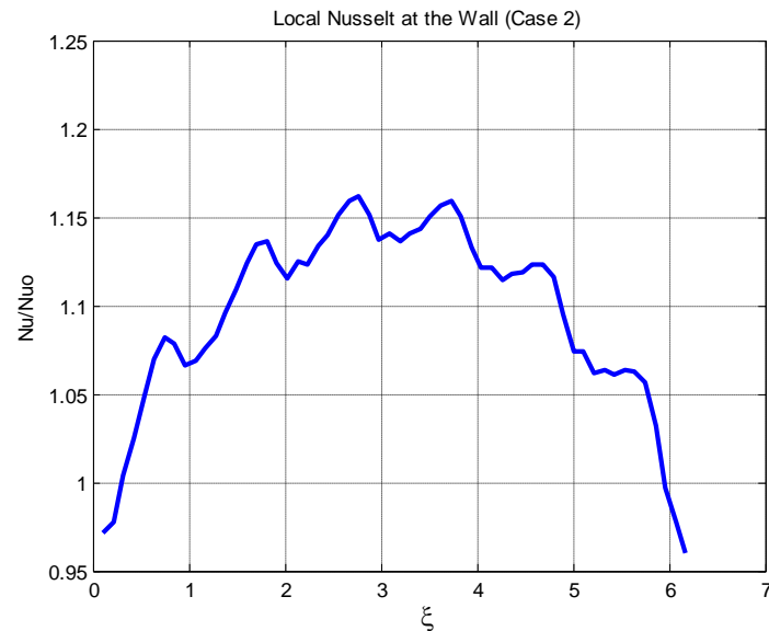
Fig7-a. Comparison of the Local Nusselt Number at the wall for the Wavy Film for the second case for Re=25 .
