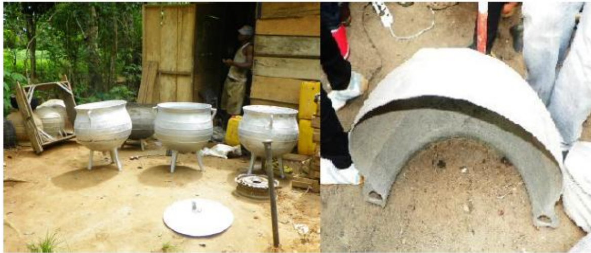
(a) (b) Plate6(a-b): Mould and Finished Products (Iron Pots)
