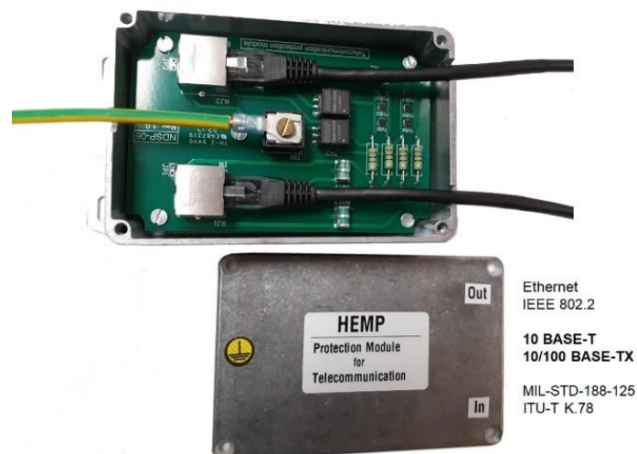
Figure15. HEMP protection module for telecommunications
