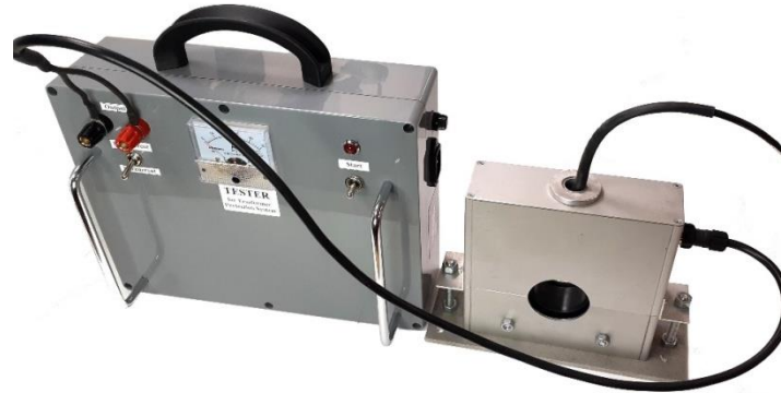
Figure11. Simple E3 component simulator for testing serviceability of the system for protection of high-power transformer
