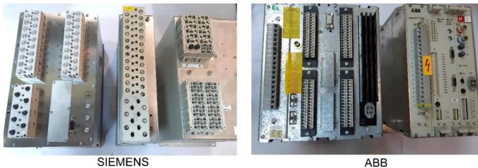
Figure2. Design of terminal assembly (connectors) of digital protection relays (DPR) or various types and from various manufacturers.
