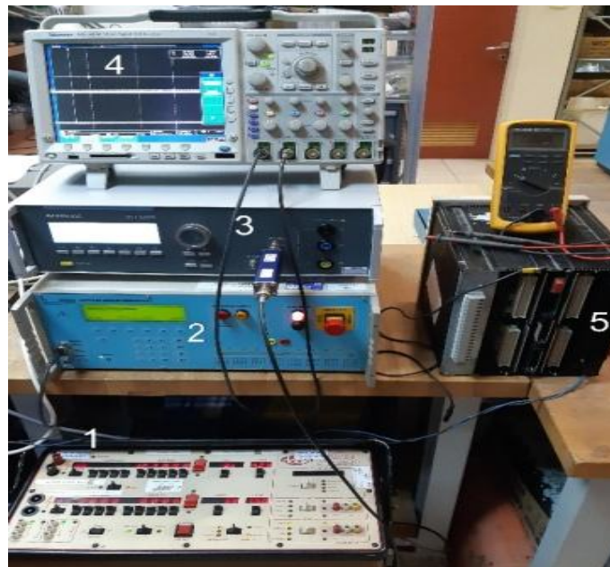
Figure1. Testing Equipment. 1 – DOBLE F2253 Simulator Of Relay Protection Modes (As An External Power Source); 2 – MIG0603 Pulse Generator; 3 – 500N EFT Pulse Generator; 4 – Tektronix MSO 4034 Pulse Oscilloscope; 5 – Test Object (Digital Protection Relay - DPR)
