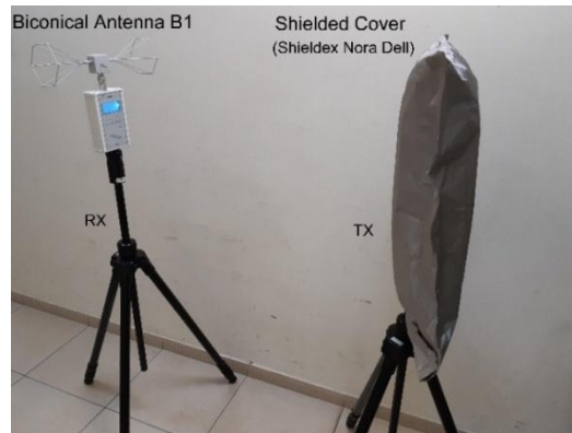
Figure 5. Measuring the shielding capacity of a case made of conductive fabric with the SEMS device.
