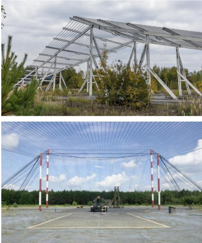
Fig4. Single port open area guided-wave simulators, produce a vertical electric field.
