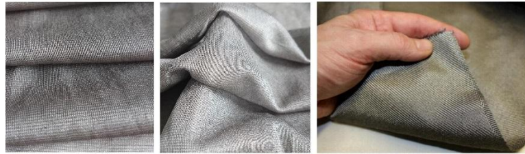
Fig4. Conductive metalized fabric to cover open parts of the cabinet's floor
