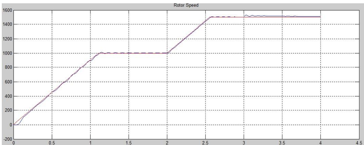
Fig11. Reference speed (red), actual speed (blue)
