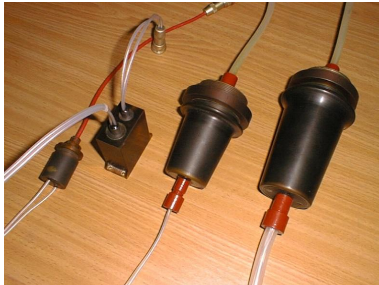
Fig6. High-voltage insulating interfaces (hercotrones) for operating voltage between input and output 10, 20, 50 and 70 kV [21].
