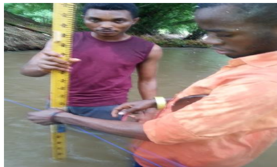
Figure2. Measuring River Depth
