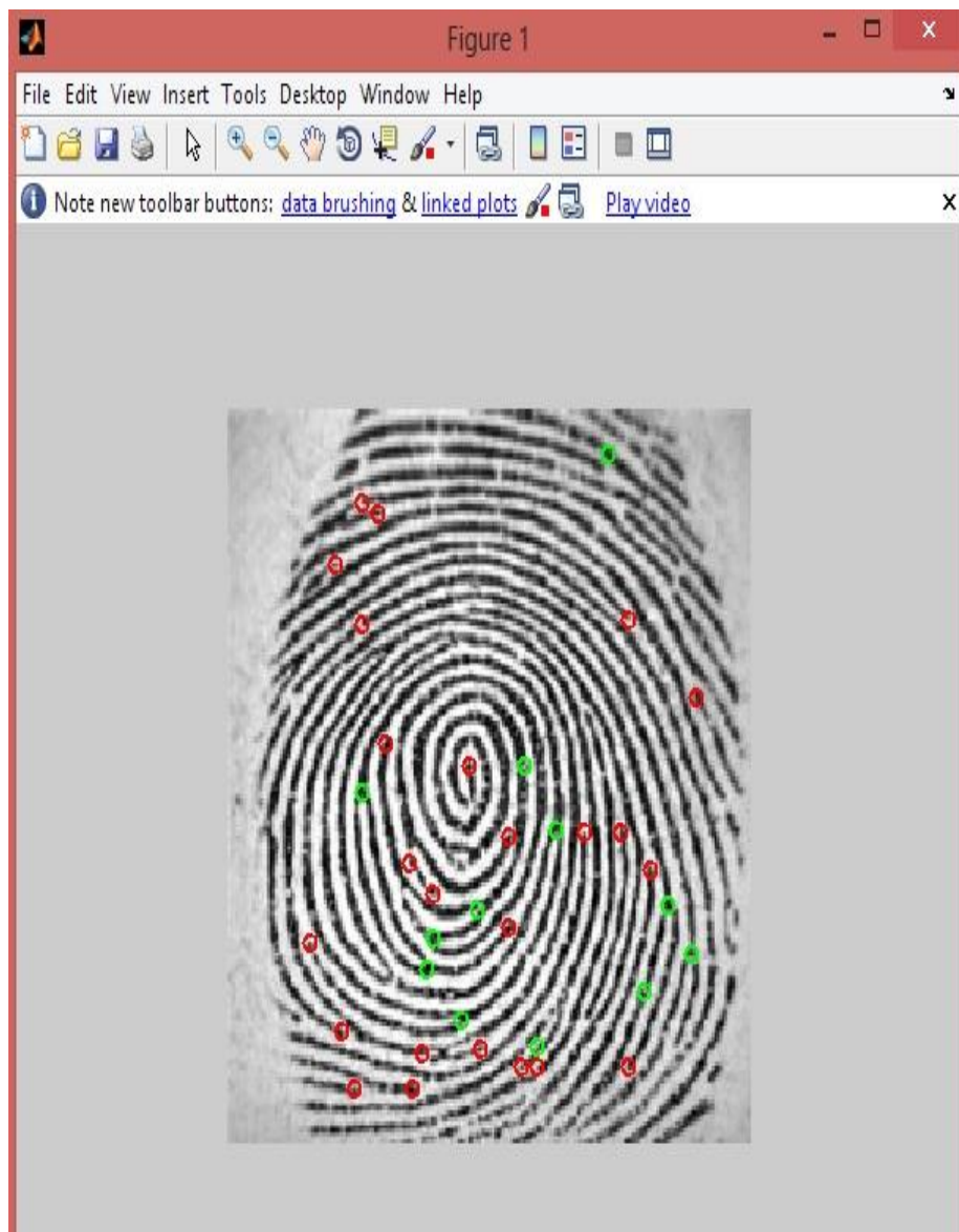
Fig8. Snapshot depicts a partially enhanced input image highlighting termination points (red colored) and bifurcations (green colored).
