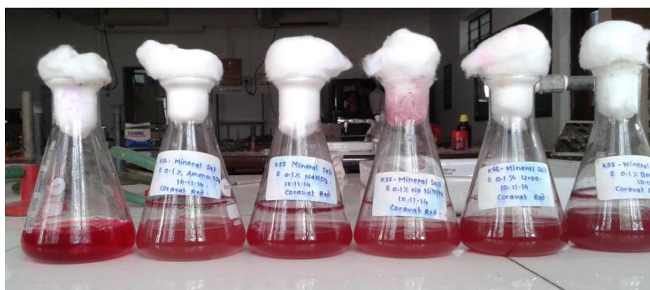
Fig3. Effect of Nitrogen source on Textile Coravat Red Dye decolourization after 24 hours
