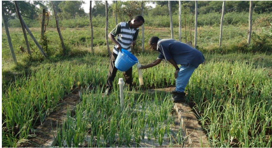
Fig1: Water application by using graduate cylinder to the Lysimeters and surrounded fields
