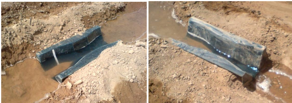
Figure 2. Providing free flow and submerged flow (right and left accordingly) when following the proper way of installation of the trapezoidal flume and when not following it.
