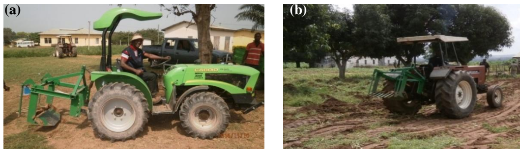
Figure 4. Harvester hitched to (a) Category I tractor (b) Category II tractor.
