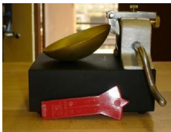
Fig 2. Showing Atterberg limit Casagrande mechanical device
