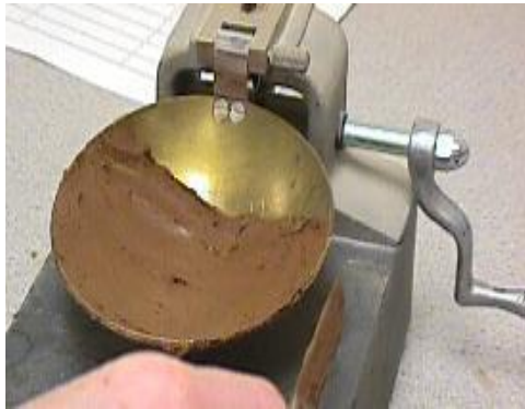
Fig 5. Experiment showing water absorbing and adsorbing ability of fine grained
