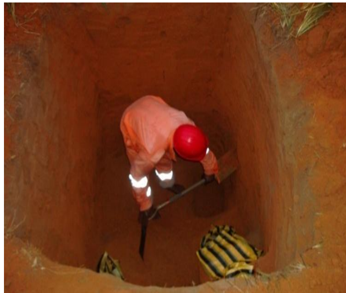
Fig 1. Showing profile pit sampling at one of the stations
