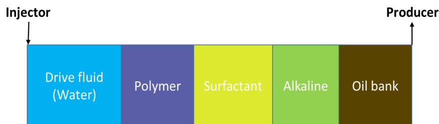
Figure9. Order in which chemicals are injected in ASP flooding
