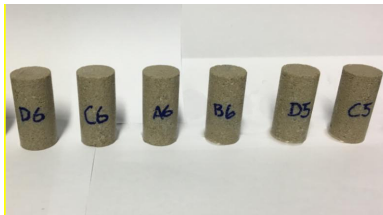
Figure6. Phase 2 core samples after flooding with brine for imitating reservoir rocks that usually have connate water.
