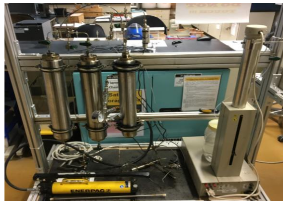
Figure5. The core flooding apparatus used for Phase2 oil flooding of cores to obtain oil permeability values
