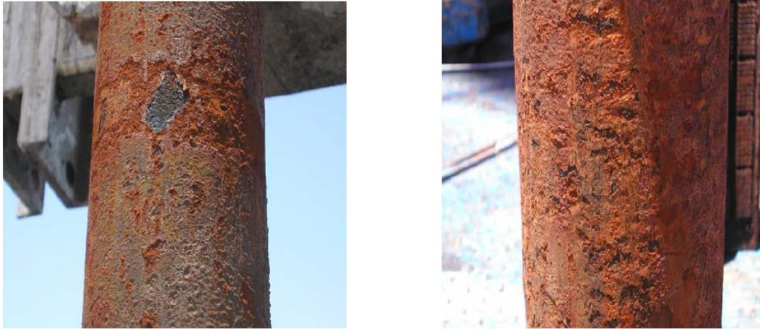
Figure5. Corrosion of S135 drill pipe (courtesy of Meng, Wan & Chen 2005)
