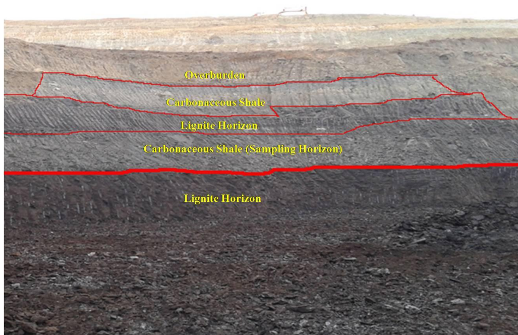
Fig2. Field photograph of the shale and lignite horizons exposed in the Surkha lignite mine
