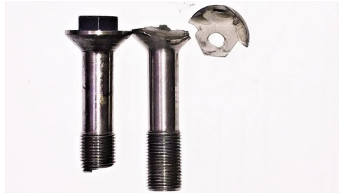
Fig7. Types of bolts fracture.
