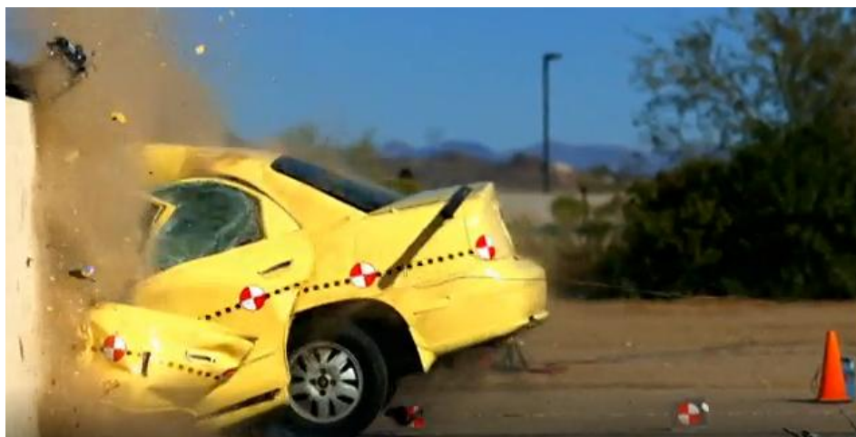
Figure8. Deformation of car at 100mph at impact as tested by Myth Busters
