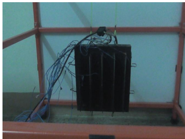
Figure2. Plain Plate with Vertical Fins Blackened Surface
