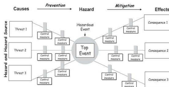
Fig1. Bowtie Measures to control threats (Prevention) and measures to control escalation (mitigation) [35].
