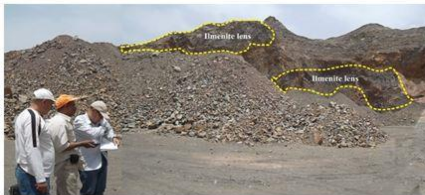
Fig3. Photograph showing the occurrence of the black type of the ilmenite ore as elongated lenses in Abu Ghalaga mine, SED, Egypt
