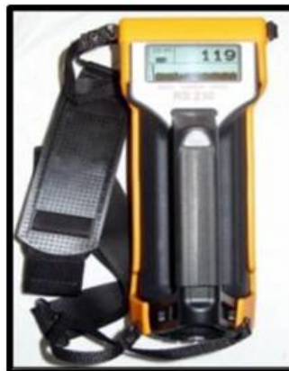
Fig. 10 Photograph showing portable gamma-ray spectrometer model RS-230
