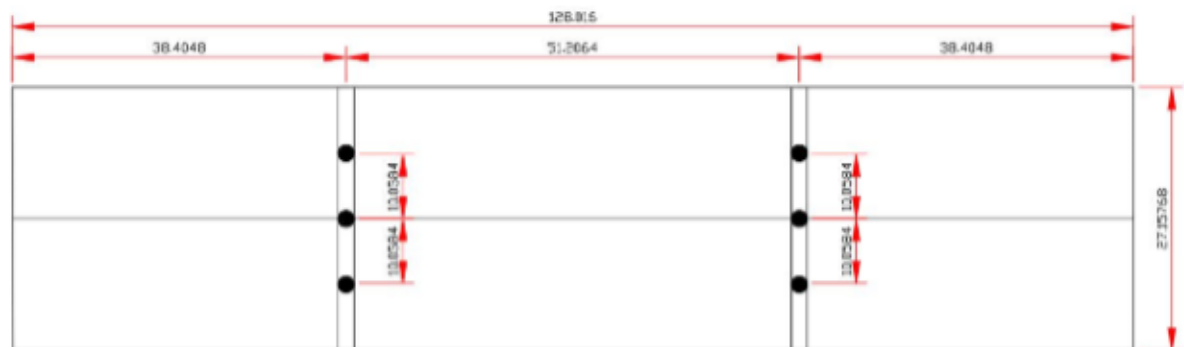
Figure2. Deck section (unit based on meters) {Mohamed A. Moustafa& Khalid M. Mosalam 2015} [12]
