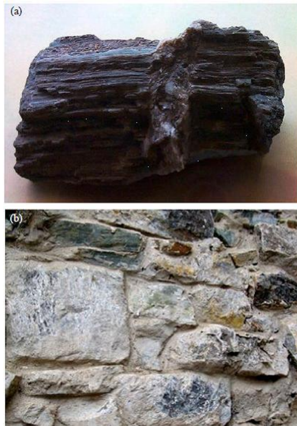
Fig1. Artificial material and its natural analogue: a) the crack of pushing in layered sandstone filled with feldspar and b) old masonry (Germany)
