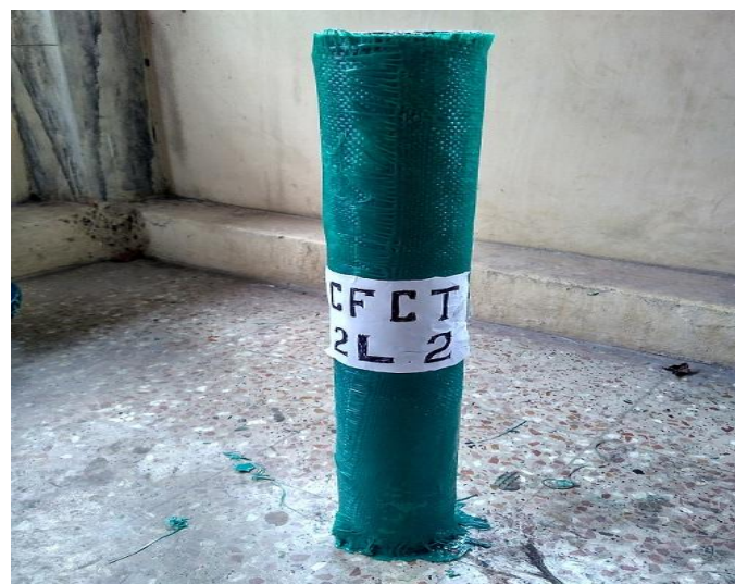
Figure8. Second layer of CFCT specimen
