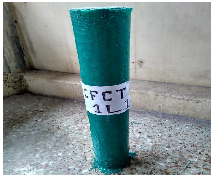
Figure7. First layer of CFCT specimen
