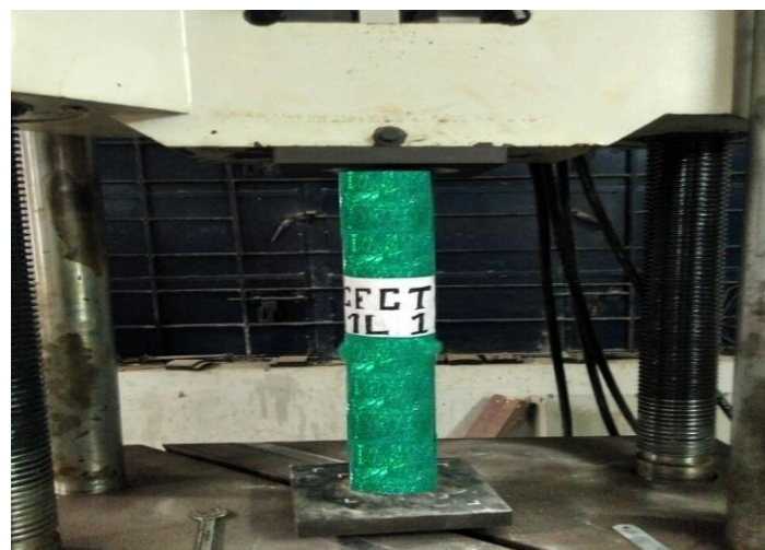
Figure11. Failure for First layer of CFCT specimen
