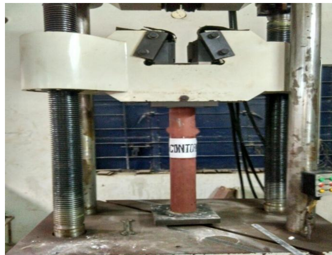
Figure10. Failure for control specimen
