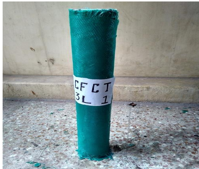
Figure9. Third layer of CFCT specimen
