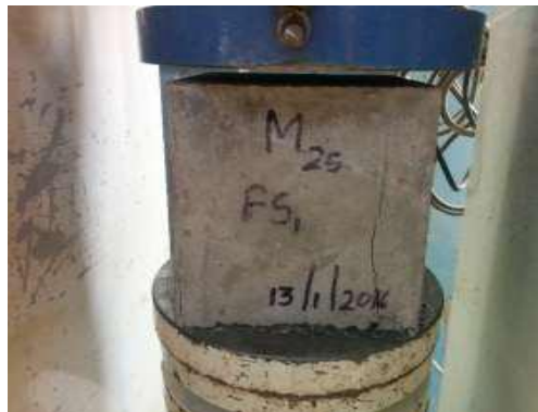
Figure1. Cracked Sample after compression test placed in UTM machine
