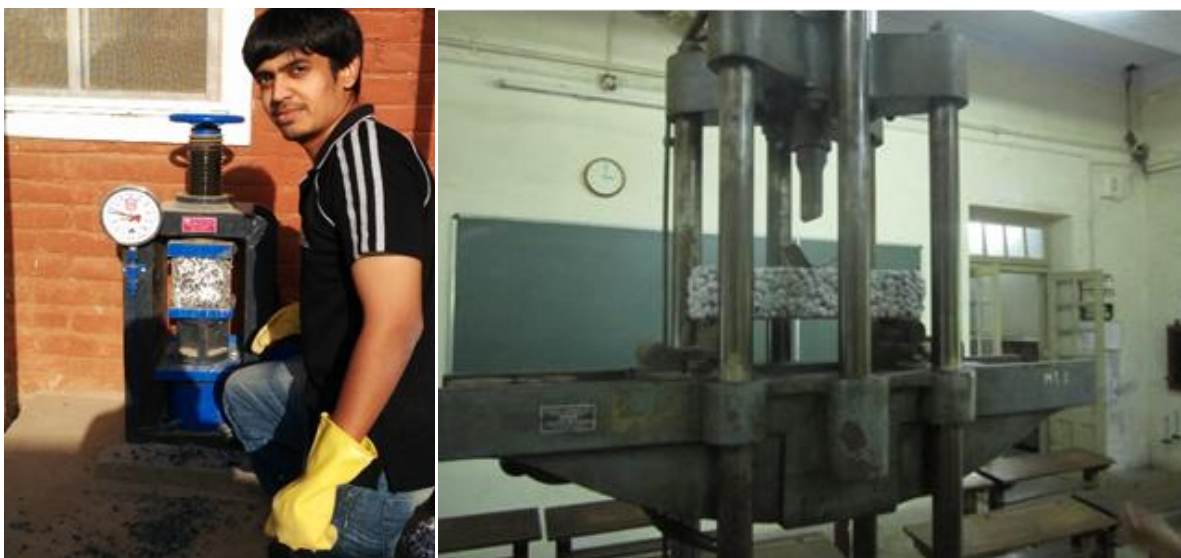
Figure3. Testing of Pervious Concrete
