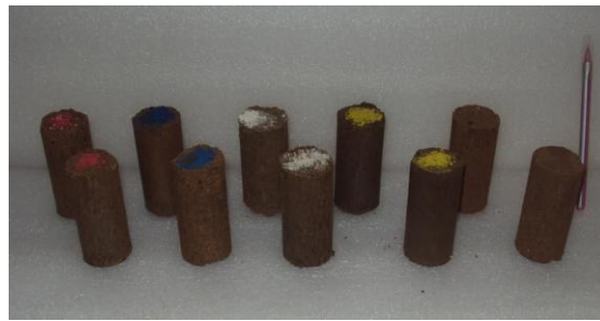
Fig4. Prepared UCC test samples at different percentage of alkali activated geo-polymers
