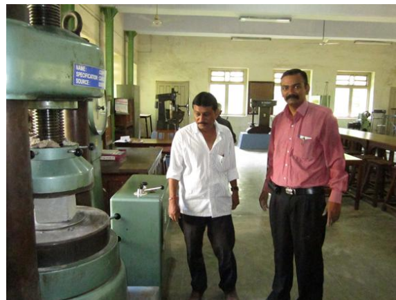
Fig.1. Setup of Compressive Strength Test
