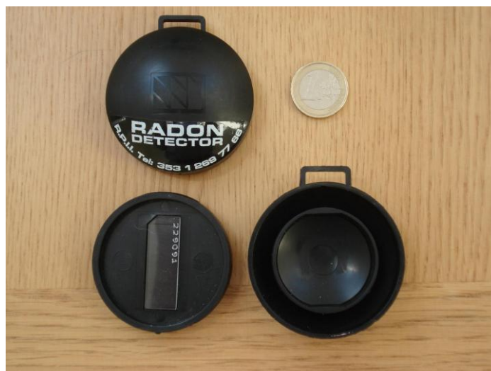
Figure4. NRPB Radon chamber structure with different parts of it.
