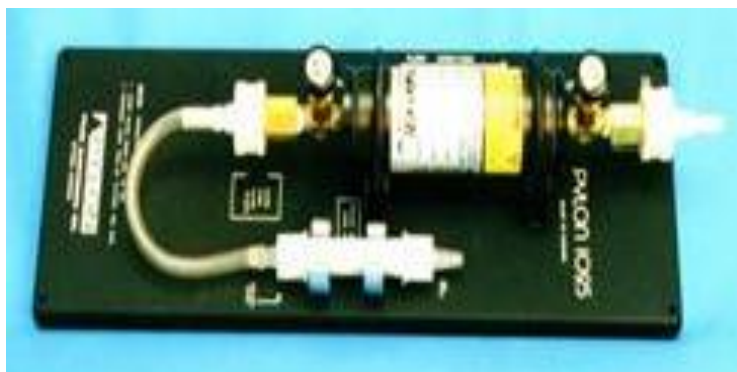
Figure1. Standard radioactive source RN-1025
