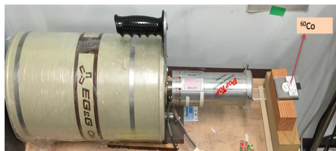
Figure1. Experimental Set-up for Ge detector
