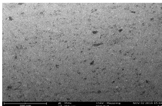
Figure1. Micrograph of corroded mild steel surface in HCl with citrus sinensis leaves extract.
