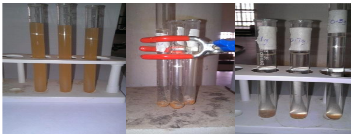
Figure 5. Coagulation actions of Alum crystals at 70°C and 25°C
