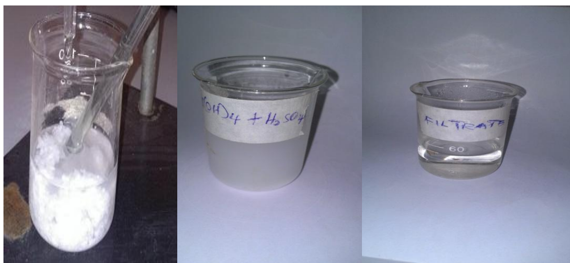
Figure 2. Formation of Aluminate ion complex
