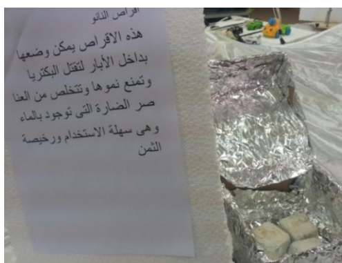
Fig3. Showing disk of silver nano particle and ceramic powder
