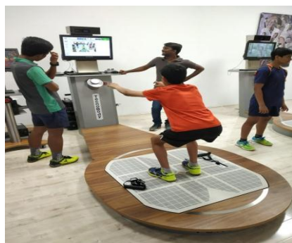
Figure2 and 3. BAI players using the Iso Lift system for assessment of Squat Jump
