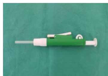
Fig (2-A): A manual propipetter used for loading of embryo into a catheter and release of the embryo into mare's uterus
